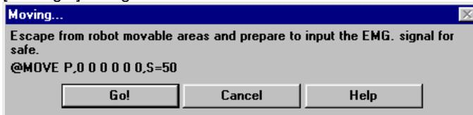
Click [Go!] button to start moving. [Go!] button changes to [Stop !] button while moving to stop axes.
