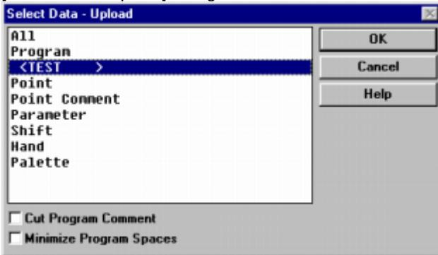
A list of data contained in [File Editor] window is shown. Select data to restore to the specified robot controller and click [OK] button.
