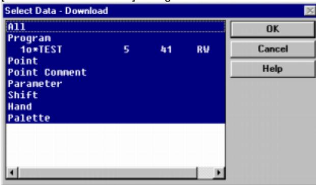
A list of data contained in the specified robot controller is shown. Select data to backup to [File Editor] window and click [OK] button.
