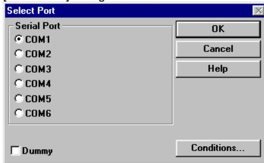
Select serial port where a robot controller is connected and select communication conditions using [Conditions...] button. Then click [OK] button.
