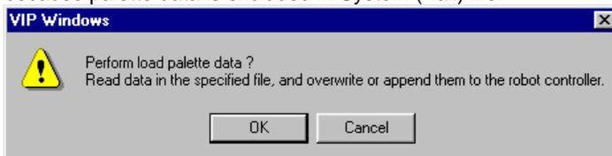
Click [OK] button if palette data is used. Otherwise, click [Cancel] button. Then, [System - Information] dialog box is shown again. Click [Close] button to return to [Robot Operate] window, and click [Close] command in [File] menu to close [Robot Operate] window.
