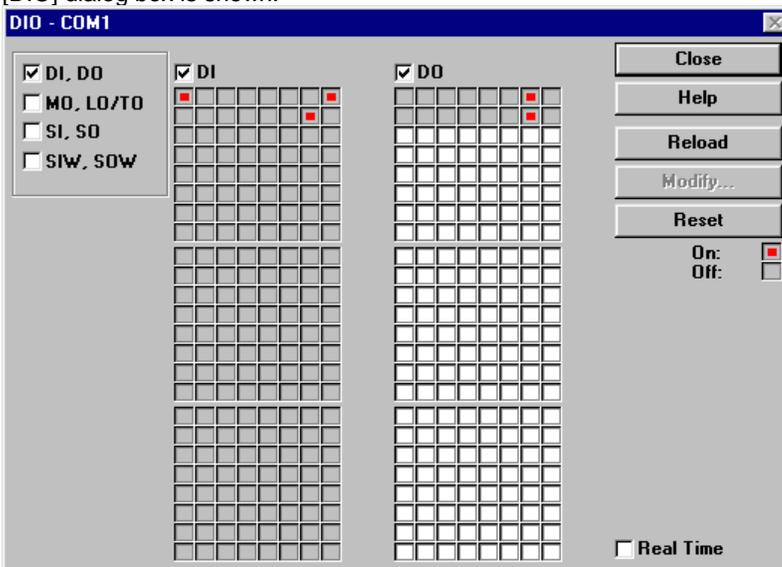
(\*) Each signal box shows robot I/O name automatically when mouse moves on box. A signal box which background colored gray shows current status. A signal box which background colored white shows current status and toggle status.
