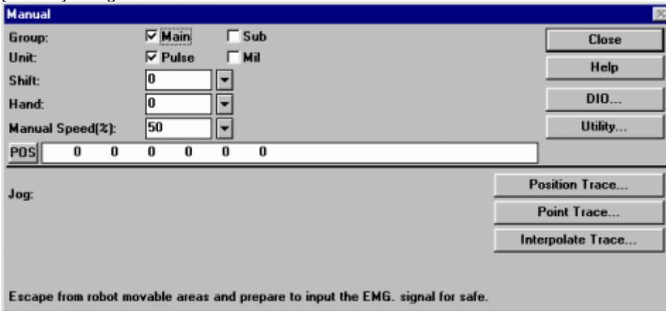
A current robot position with specified group, unit, shift coordinate and hand definition, and also manual movement speed.
