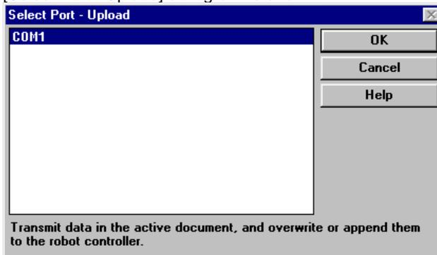
A list of serial port connected to robot controllers is shown. Select a port to restore data and click [OK] button.
