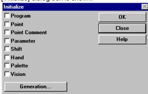
4. Check check box for each data to be initialized and click [OK] button. An initialized data cannot be recover.
